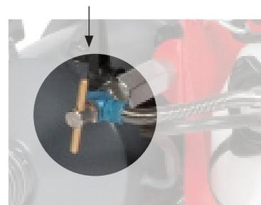
The Turbo ULV is a portable, electrically operated pneumatic cold fogger. Its high performance turbine creates a strong warm air stream of up to 50 l / s (free blowing). The formulation of biocide is atomised into a fine aerosol, which is adjustable from approx. 10 to 100 µm dependent on flow rate (nozzle size used). The precise flow regulation is provided by means of interchangeable nozzles. Nozzles and fogging conduits withstand weaker acids and bases with pH-value 5 – 9.
