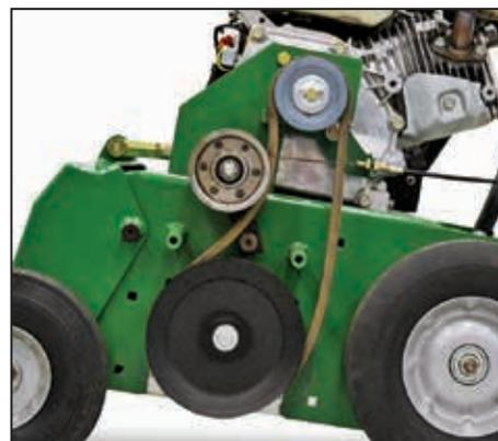
**Premium pulleys**, easy to adjust idler, and easy to change belt contribute to simple service and long life. Protected by a steel guard.
