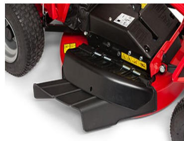
CONTROL YOUR SPEED Variable speed disc drive transmission. Easily change from mulching to side discharge.
